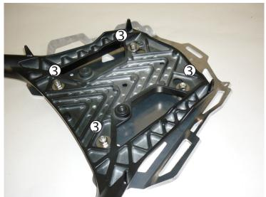
Place large M6 washer and M6 lock nut on each bolt, getting them started by hand. A dab of grease on the threads will help, and will make future disassembly easier. Using the M4 driver, hold the bolt stationary while turning the nuts to tighten. Torque each screw to 10nm.
