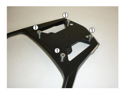
Remove the OEM rack from the bike. Remove the rubber pad to expose the underlying holes, you will not re-install it. Place the (4) spacers as shown.
